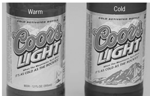
Fig. 3. Beverage label printed with a thermochromic leuco dye in their (a) colorless and (b) colored states.
